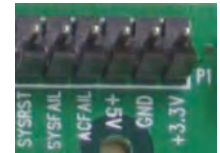
6-Pin Utility Connector On rear of Backplanes
