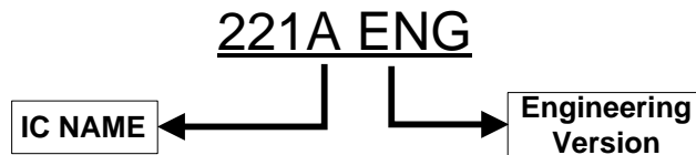
Figure 8-1 IQS211A engineer version, marked as 221A.
