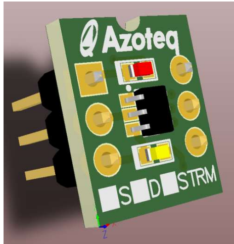
Figure 3.1 Top view of square daughter board. When looking from the top, IC and PCB pins are mapped one-to-one.
