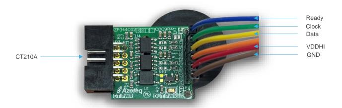
Figure 1.1: CT001 Isolation Streaming Board Connection
