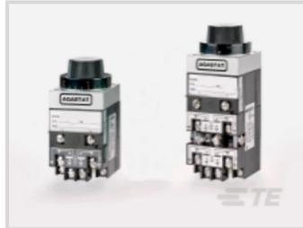
Type of Control: **Knob**Input Voltage: **120 – 110 VAC**Contact Current Rating: **10A@240VAC A**Mode of Operation: **On-Delay**Delay Time: **1 – 10 minutes**
