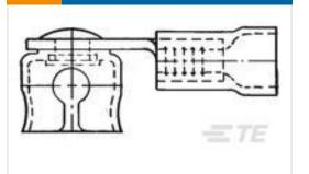
TE Part #55137-1 TERMINAL,PG TUBE CAP 22-16
