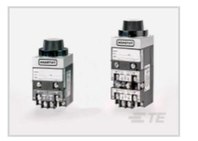
Type of Control: Knob Input Voltage: 240 – 220 VAC Timing Range (Off-Time): 20 – 200 seconds Contact Current Rating: 10A@240VAC A Mode of Operation: Off-Delay
