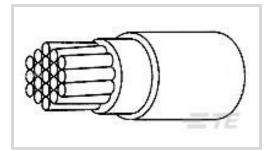
Cable Type: Spec 99M Voltage Rating: 600 V Insulation Material: Radiation-Crosslinked, Modified Polyester Conductor Material: Tin-Plated Copper Wire Size: 12 AWG
