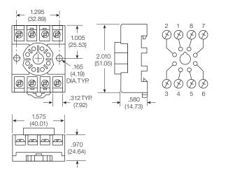
Screw terminal, DIN rail, snap-mount socket 27E892 Offers screw termination for KRPA relays and other devices with 11-pin undecal base. This socket is constructed with a spring-loaded latch which allows it to be quickly snapped
