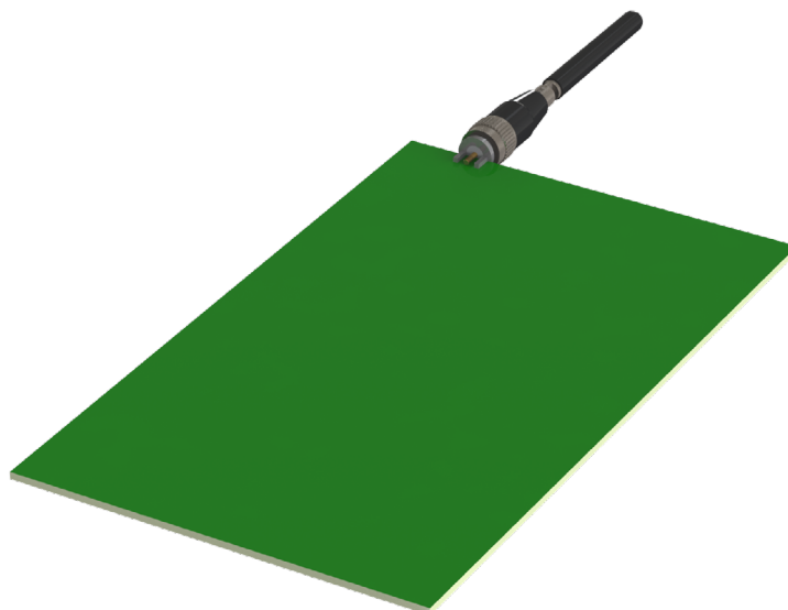
Figure 17. ANT-W63-MON-ccc on Edge of Ground Plane, Bent 90 Degrees (Edge-Bent)
