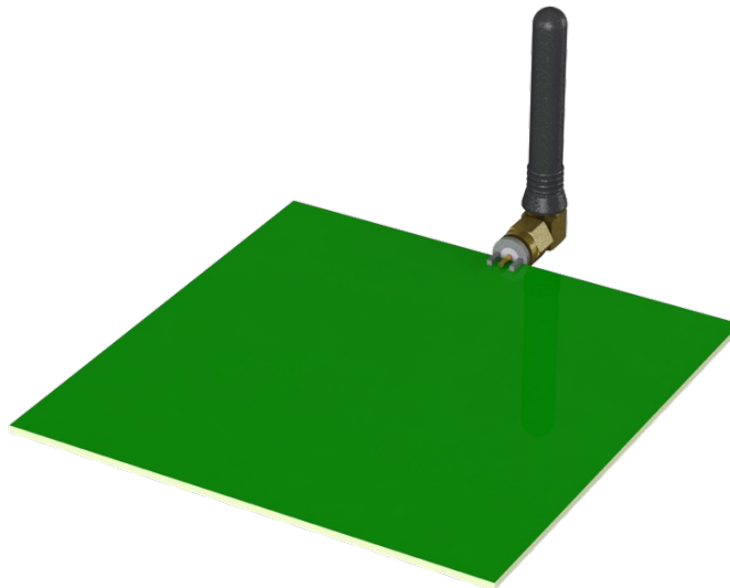
Figure 10. ANT-W63-CW-RCS-ccc on Edge of Ground Plane
