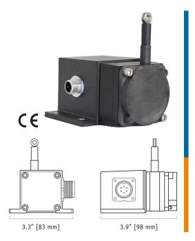
The PT1MA adds 4...20 mA position feedback signal to Celesco's compact line of cable-extension transducers. The PT1MA is available with full stroke ranges from as little as 2 inches on up to 50 inches with adjustable zero and span settings to precisely match the full scale output to your exact measurement range.
