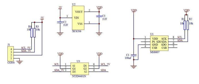
Connector Pin Assignments (I<sup>2</sup>C Communications)
