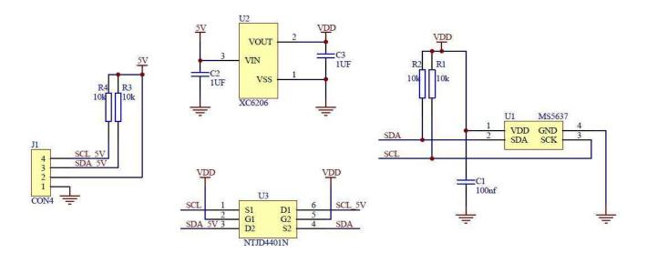
Connector Pin Assignments (I<sup>2</sup>C Communications)
