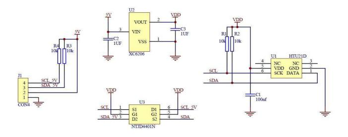
Connector Pin Assignments (I<sup>2</sup>C Communications)
