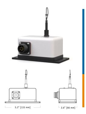
The DPT250 Cable-Extension Transducer offers a highly accurate incremental encoder output signal that can provide both position and velocity information. The output is a digital pulse stream that can provide resolution down to less than a thousandth's of an inch!
