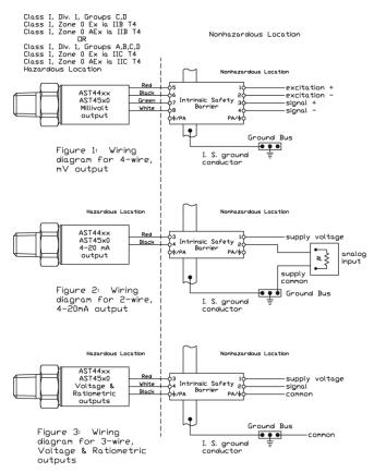
The transducers listed below are designed for installation in EITHER Class I, Division 1, Groups C.D.; Class I, Zone 0 Group IIB DIR Class I, Division 1, Groups A,B,C,D.; Class I, Zone 0 Group IIC hazardous locations when connected to Associated Apparatus as described in note 1.
