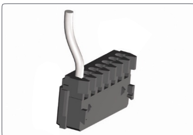
Unstripped wire inserted into MT housing.
