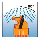
Protected against spraying water (up to 60° inclination)
