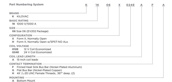
(2) User furnished bus bar must be equivalent to 4X 4/0 conductor. Torque to 45-55 in-lbs. per connection (5.1 - 6.2 NM)
