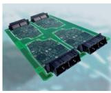
PCB and connectors are loaded manually into fixtures. When started, the machine checks the correct loading of the connectors before placing the connectors onto the PCB. The tool then moves under the press ram where the connectors get pressed one after the other onto the PCB. The CBP-5T servo-electric press is used to seat the PCB which provides a force-distance check to guarantee quality production.
