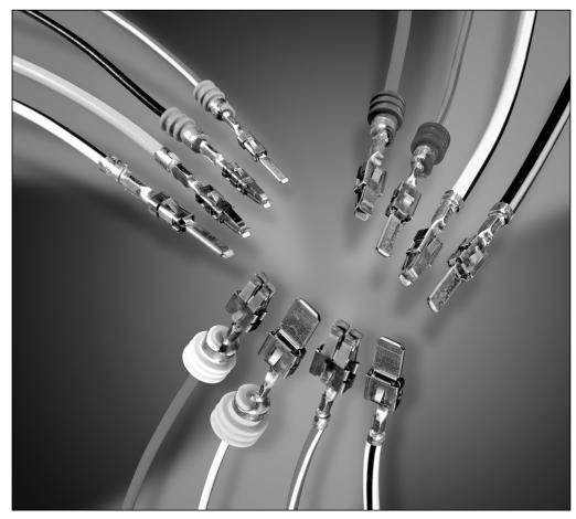
The receptacle contact has two, respective four contact springs, which are independent of each other and a steel top spring.
