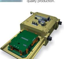
A special tooling plate allows the sequential pressing of a number of different pre-loaded connectors. An intermediate plate, positioned between the PCB with its pre-positioned
