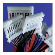
The IDC workstation produces electrical connections for harness assemblies specifically intended for the use within dashboard applications in the automotive industry. The proven insulation displacement technology ensures a high level of reliability. The software allows the
