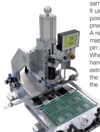
The P50 Insertion machine is a manual operated bench machine for low volume production, repair work and sample production. It uses a trader slide to position the PCB under the pneumatic insertion head. A regular PCB is used as master to position the indexing pin above the insertion hole. When activating the two hand start, the indexing pin extracts. If a hole is detected, the terminal is inserted into the board in production.
