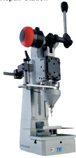
A loose-piece pin or tab is placed in the product specific insertion finger of the arbor press, the PCB is placed on the support anvil and the pin or tab is manually pressed into the board.
