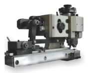
The FFC Applicator is designed for FFC and FPC terminations. It is normally delivered with a special TE Connectivity crimp machine, but is also compatible with standard presses (press stroke 40 mm), if a wire feed is supplied. The adjustment of the crimp height is similar to other TE Connectivity crimp applicators. All wear parts are easy to change. The FFC Applicator is available for different TE Connectivity contacts, such as:
