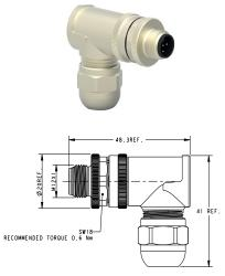
All dimensions in mm. Temperature range: -40 to +85° C. Products can also be obtained with silver-plated contacts upon request.
