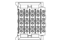
Part Number 5120742 30 Position Center Header Feed-Through
