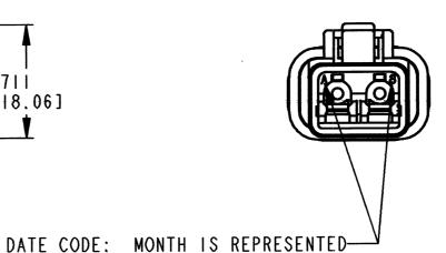
MODIFICATION: PLUG IS BLACK, GROMMET IS AN E-SEAL, SHRINK BOOT.
