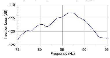
The plot at left shows an estimate of the frequency response curve for two identical units, one driven as transmitter, the other acting as a receiver. The spectrum of the received signal was divided by that of the drive signal and gain stage, giving the overall insertion loss as a function of frequency (measured at 30 cm distance, in air).
