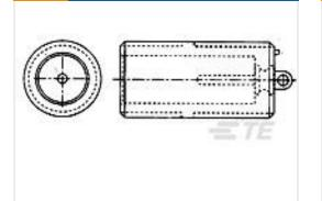
TE Model / Part #448463-1 LGH-1 RCPT,W/1/2-32 UN THREAD
