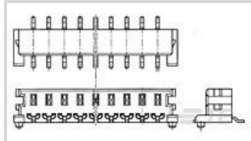
PCB Connector Assembly Type: **PCB Mount Header**PCB Mount Orientation: **Right Angle**Connector System: **Wire-to-Board**Number of Positions: **11**Centerline (Pitch): **1.5 mm [.059 in]****Features****Product Type Features**
