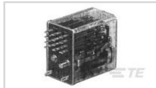
Power Relay Type: **Industrial Panel Plug-In**Coil Magnetic System: **Monostable, DC**Coil Power Rating Class: **150 – 200 mW**Coil Power Rating DC: **175 mW**Coil Resistance: **1000 Ω**
