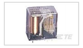
Contact Voltage Rating: 125 VAC Signal Relay Coil Power Rating (DC): 647 mW Signal Relay Mounting Type: Printed Circuit Board Signal Relay Terminal Type: Plug-In, Solder
