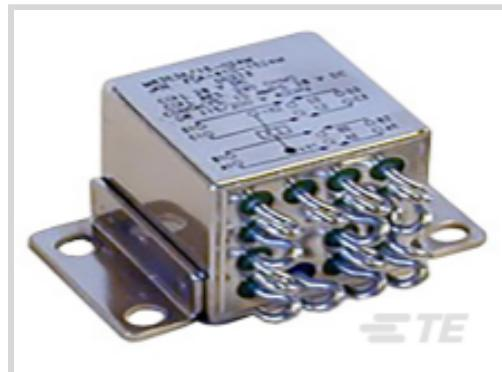
Mid-Range Relay Contact Arrangement: **4 Form C, 4PDT, 4 C/O**Coil Suppression Diode: **With**Auxiliary Contacts: **Without**Terminal Plating: **Tin-Lead**Mid-Range Relay Contact Current Rating: **10 A**
