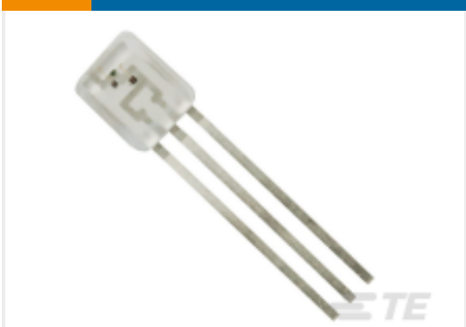
TE Part #11032254-00 EMITTER 660/940NM 1 2
