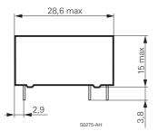
Datasheet Rev. GH1 Issued 2007/08 www.tycoelectronics.com www.schrackrelays.com Dimensions are in mm unless otherwise specified and are shown for reference purposes only. Product specification according to IEC 61810-1. Product data, technical parameters, test conditions and
