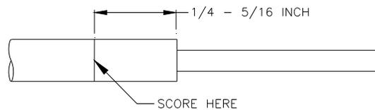
5. Remove section of jacket carefully by pulling straight. This will flatten the braid strand ends.
