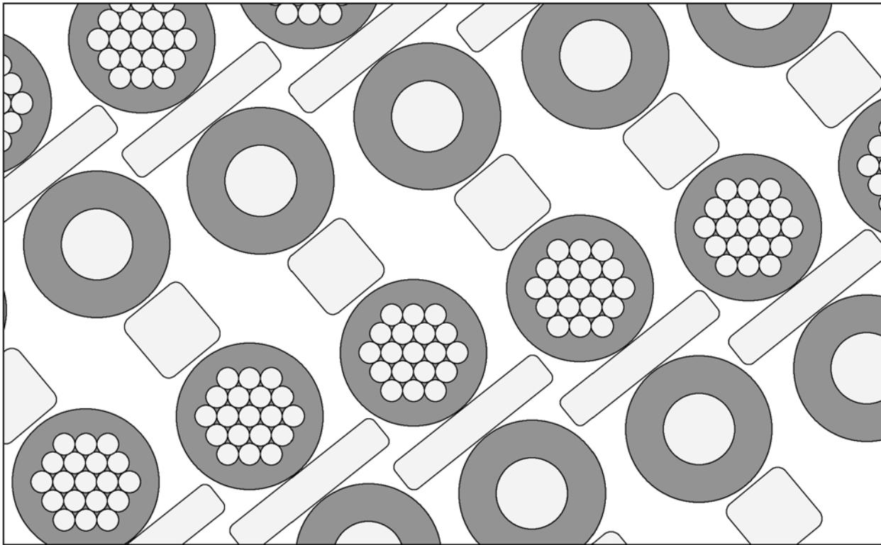
For best results, the proper terminal or splice must be selected not by the "fit" of wire or wires in the terminal barrel, but by the total circular mil area in cross section of the wires used. For this purpose convenient tables have been prepared to assist in the calculation of circular mil areas. When the totals are known, the proper terminal or splice can be determined quickly.
