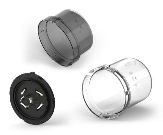
THE BASE ASSEMBLY INCLUDES POWER TWIST LOCK TERMINALS, SPRING LEAF SIGNAL TERMINALS, AND AN INTEGRAL SEALING GASKET. COUPLE THAT WITH AN IKO8 RATED COVER AND THE ASSEMBLED NETWORK LIGHTING CONTROL ACHIEVES AN IP66 SEAL RATING.
