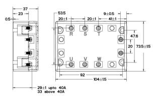
\* Overall height dimensions includes with clear cover Dimensions in mm
