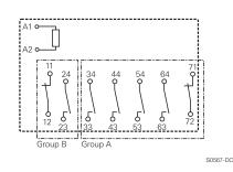
**Product code structure** Typical product code SRL 7 52 3 D 024 Type SRL Relay with force guided contacts SRL Version 7 pole **Contact arrangement 52** 5 form A + 2 form B contacts (5 NO + 2 NC) **Contact material** 3 Ag SnO Coil system **D** DC coil Coil Coil code: please refer to coil versions table (e.g. 012=12VDC)
