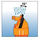
Protected against vertically dripping water when tilted up to 15°
