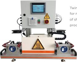
Twin workstation heater for multiple installation of short length tubing products
