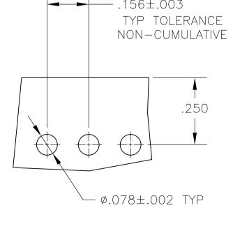
FOR MOUNTING HEADER FLUSH TO BOARD EDGE
