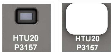
Laser marking on HTU20P(F) sensor
