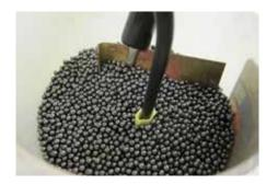
Figure 6 - Dielectric Strength Test - PLASTI-GRIP Terminal
