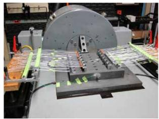
Figure 3 - Military Vibration Test - PIDG Terminals
