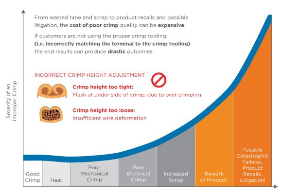
Cost of an Improper Crimp
