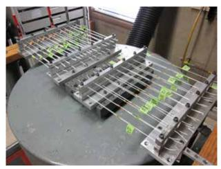
Figure 2 - Military Vibration Test - SOLISTRAND Splices
