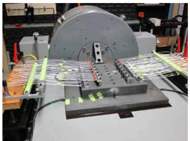
Figure 3 – Military Vibration Test - PIDG Terminals
