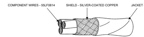
JACKET - LOW OUTGASSING, ULTRA LOW FLUORIDE, RADIATION-CROSSLINKED, MODIFIED ETFE
