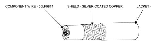
JACKET - LOW OUTGASSING, ULTRA LOW FLUORIDE, RADIATION-CROSSLINKED, MODIFIED ETFE
