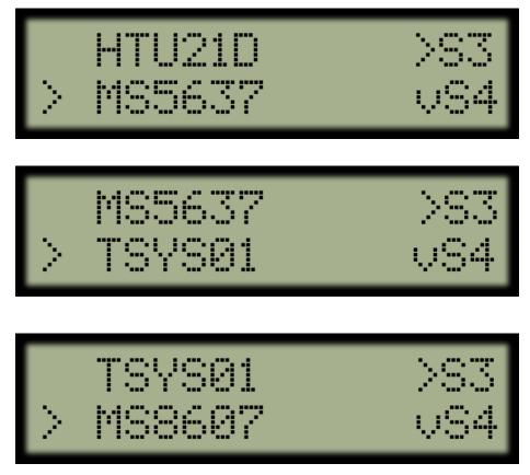
Then press S3 to select the desired sensor and start its measurements.
