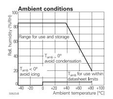
NOTE: For use conditions the temperature limits as indicated in the datasheets apply.
